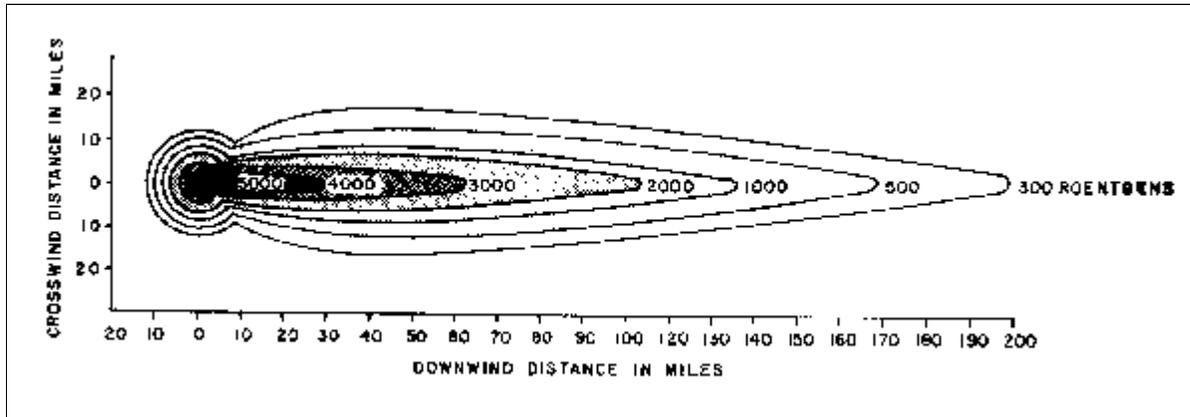
This was the fallout pattern 36 hours after a single 15-megaton thermonuclear device (the Bravo shot of Operation Castle at Bikini Atoll - March 1, 1954) was detonated. The eventual extension of the fallout was more than 20 miles upwind and over 320 miles downwind. The width in cross section was variable, the maximum being over 60 miles. This means there was substantial fallout contamination over an area of more than 7000 square miles.
